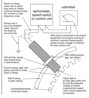
$f_{output} = \frac{\text{engine R.P.M. x no. of flywheel teeth}}{60}$
